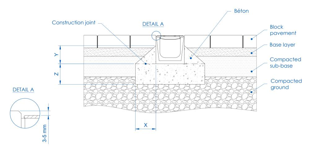
\* In case of an incorrect compactation of the soil, the concrete embracement must be made up to the pavement level.
